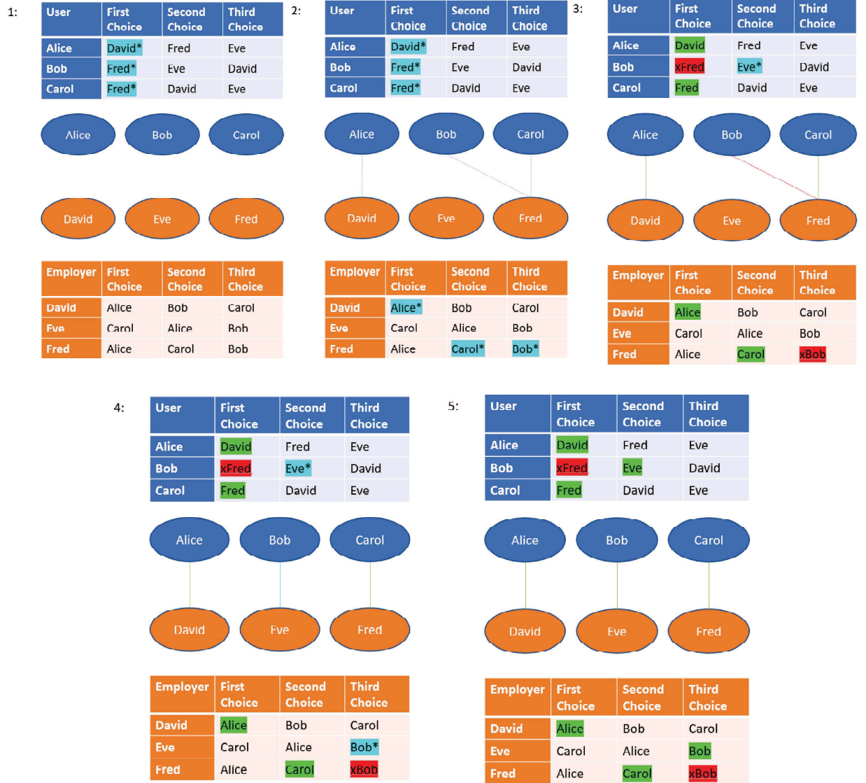
Figure 6: An example of running the modified Gale-Shapely algorithm
