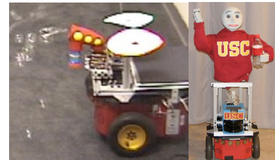
Figure 1: Left: The mobile robot used in the experiment. Right: The humanoid robot used in the experiment.
