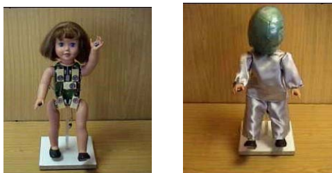
Figure 1: The robot used in the trials. The figure on the left shows the 'undressed' version revealing the robotic parts that control its movement. On the right we see Robota with a face mask and costume (see [14] for a detailed investigation about the robot's appearance).
