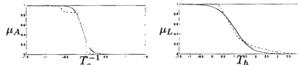
Figure 4: Actual (dashed line) and approximated (solid line) membership functions: (a) accuracy and (b) liability.
