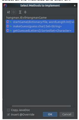
IntelliJ will automatically generate the needed code
